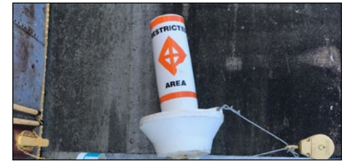
A plastic buoy and counterweight at Lock and Dam 9, near Lynxville, Wisconsin. USACE courtesy photo
